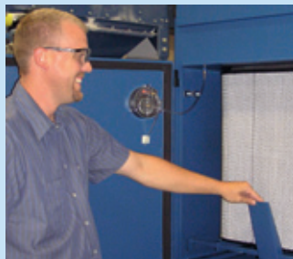
One pivot lever securely retains the primary filter element
